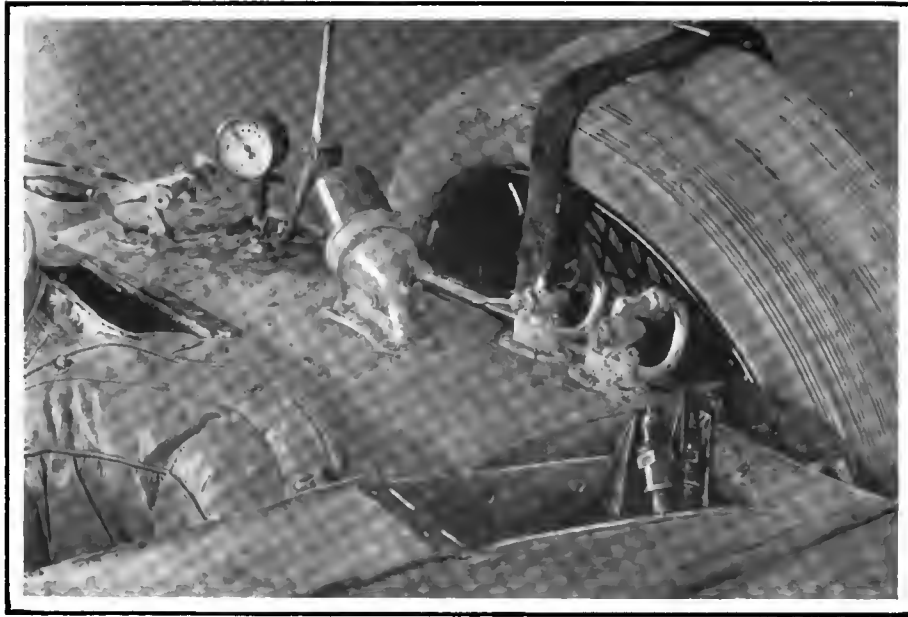
Fig. 4—Rear end of Mercedes racer showing gasoline tank mounted transversely together with various tool-carrying compartments around the tank. At the left side is a compartment for spare spark plugs and other articles. At the right is a compartment for the thermos bottle. In the center are two spaces for jack and jack lever
